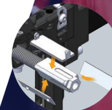
Keeping the scope rod close to the elevation rail - The key to stability
