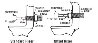
**Centerest Flipper**<sup>®</sup> can be adjusted left or right of center as needed for optimum arrow flight (1/4 Turn = 0.01"). It is ideal for hunters since it can be replaced instantly in the field without affecting original sight settings.
